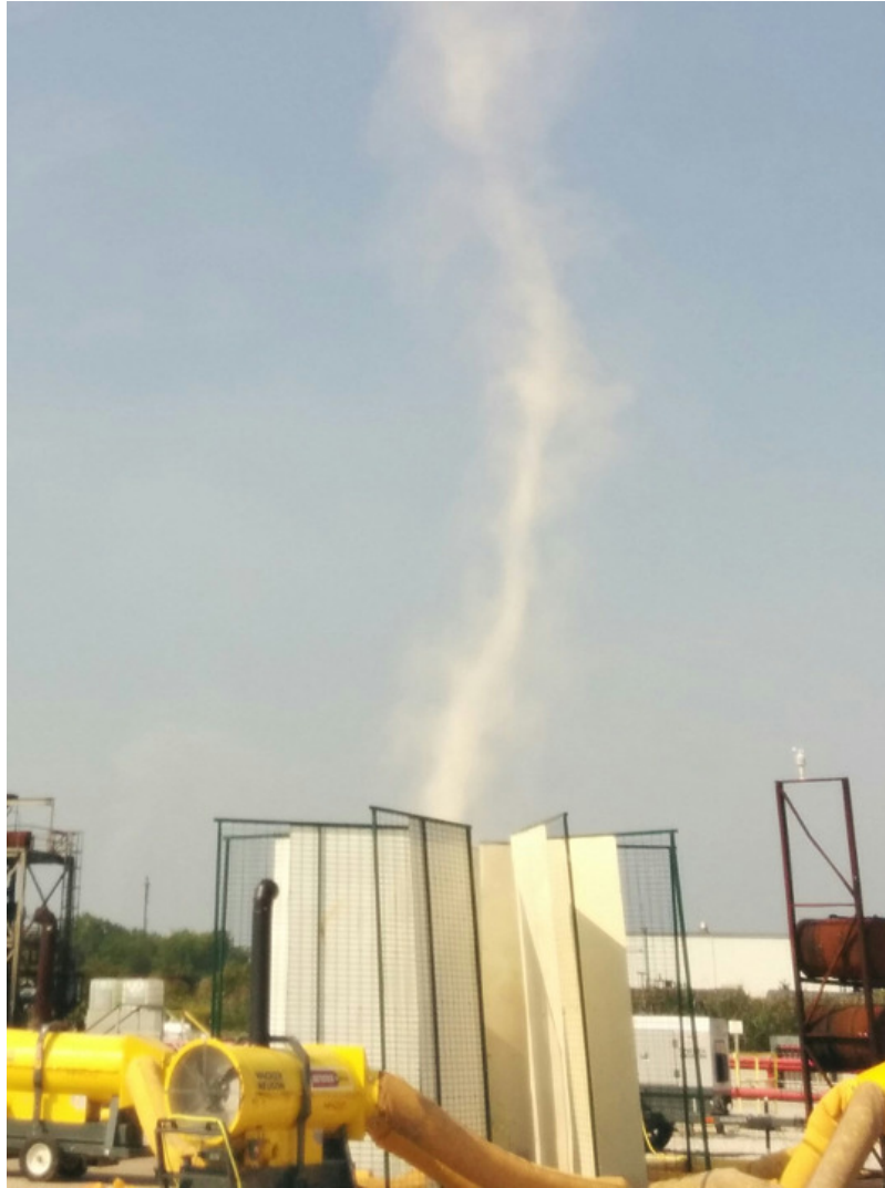
Fig. 4 Unenclosed Prototype – Vortex made visible with white smoke emitter
