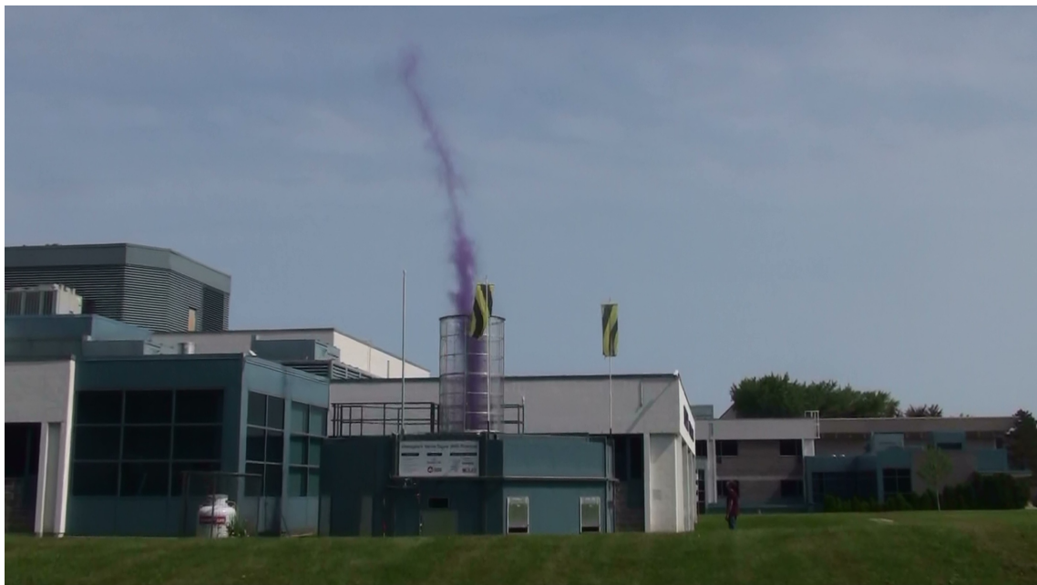
Fig. 2 Enclosed prototype vortex made visible with black smoke emitter
